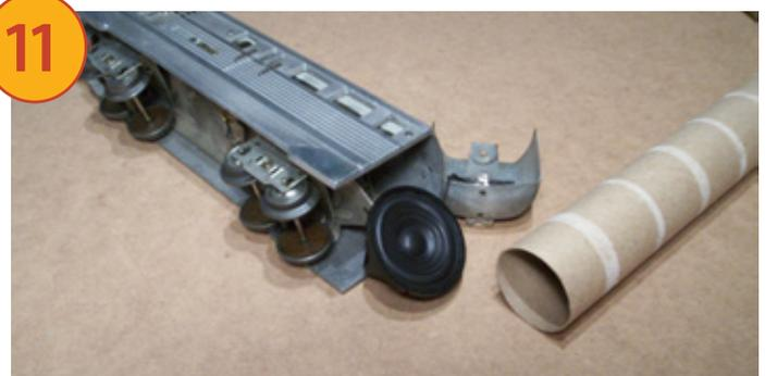
**The speaker for** RailSounds is tucked into the rear of the baggage/coach car. Not an ideal spot, but as you can see from the opening in the shell, there isn't much space to work with because of a high sheet-metal floor and a central-mounted bulb that illuminates the car. I used a cardboard tube to make a sound box (as per the instructions that came with the RailSounds installation kit) to improve audio quality. After that, I tested my installation, and the TMCC *Zephyr* was ready to roll.
