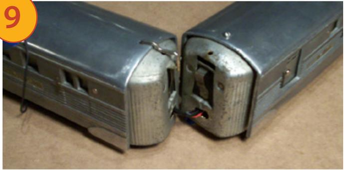
**After installing the** RailSounds boards in the front of the baggage/coach car (again up against the roof of the shell), I took a deep breath and made the only non-reversible modification to my *Zephyr* – cutting oval-shaped holes in the two vestibules for the six-pin tether connecting the RailSounds and TMCC boards. The holes are at the lower edge of the vestibules (you can see the red wire).
