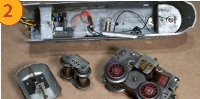
**When disassembled,** there seems to be plenty of room for the TMCC/RailSounds components. However, looks can be deceiving. The TMCC boards here are temporarily placed in the rear of the power car's shell. The motor-and-drive mechanism takes up most of the space in the center of the shell. A cast-in rear brace, sheet-metal light-bulb brackets, and stamped-metal vestibule eat up a lot of real estate on this model.
