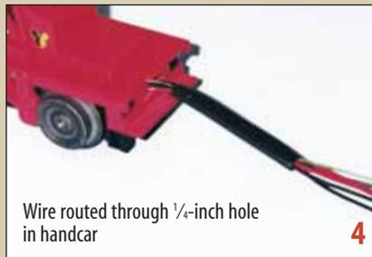
ter-rail roller to carry current to the motor in my handcar. I wanted the resulting “trailer” to look as charming as the original, so I used the truck as a basis for a tiny ore car built from .060-inch sheet styrene. And wouldn’t you know it, the ore car also provided just enough space for me to add a Lionel no. 600-0103-001 electronic reverse unit and a lock-out switch.
